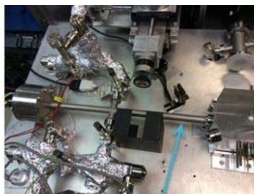
Time-of-flight tube: The ion source is at the right-hand end and the detector at the left. This image is a closer view of the bottom right of the previous image
