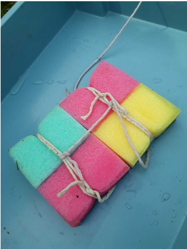
Figure 15 – Assembling the colonising media
