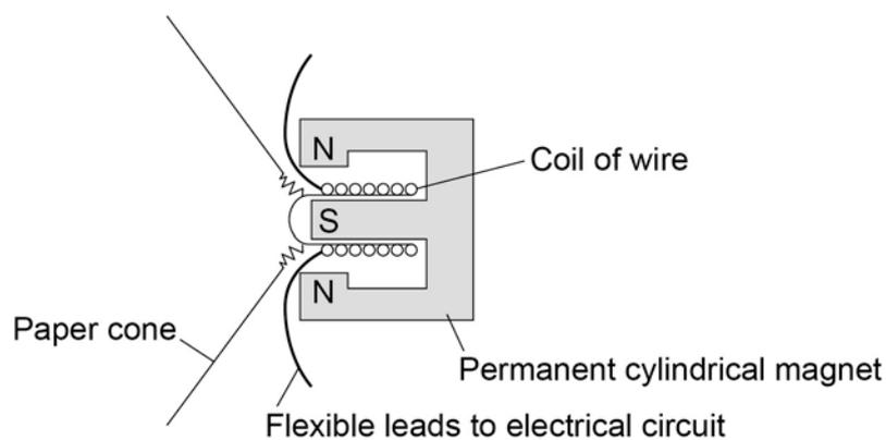
Explain how the loudspeaker converts current in an electrical circuit to a sound wave.
