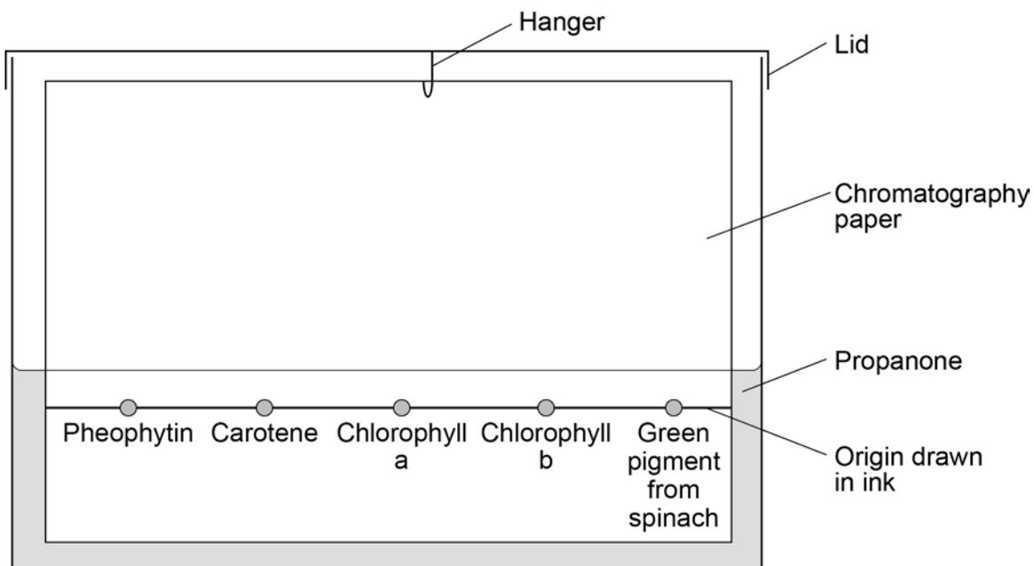
This student did not set up the apparatus correctly.
