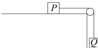
The block  $P$  has mass  $0.4 \text{ kg}$  and the coefficient of friction between  $P$  and the surface is  $0.5$ .
