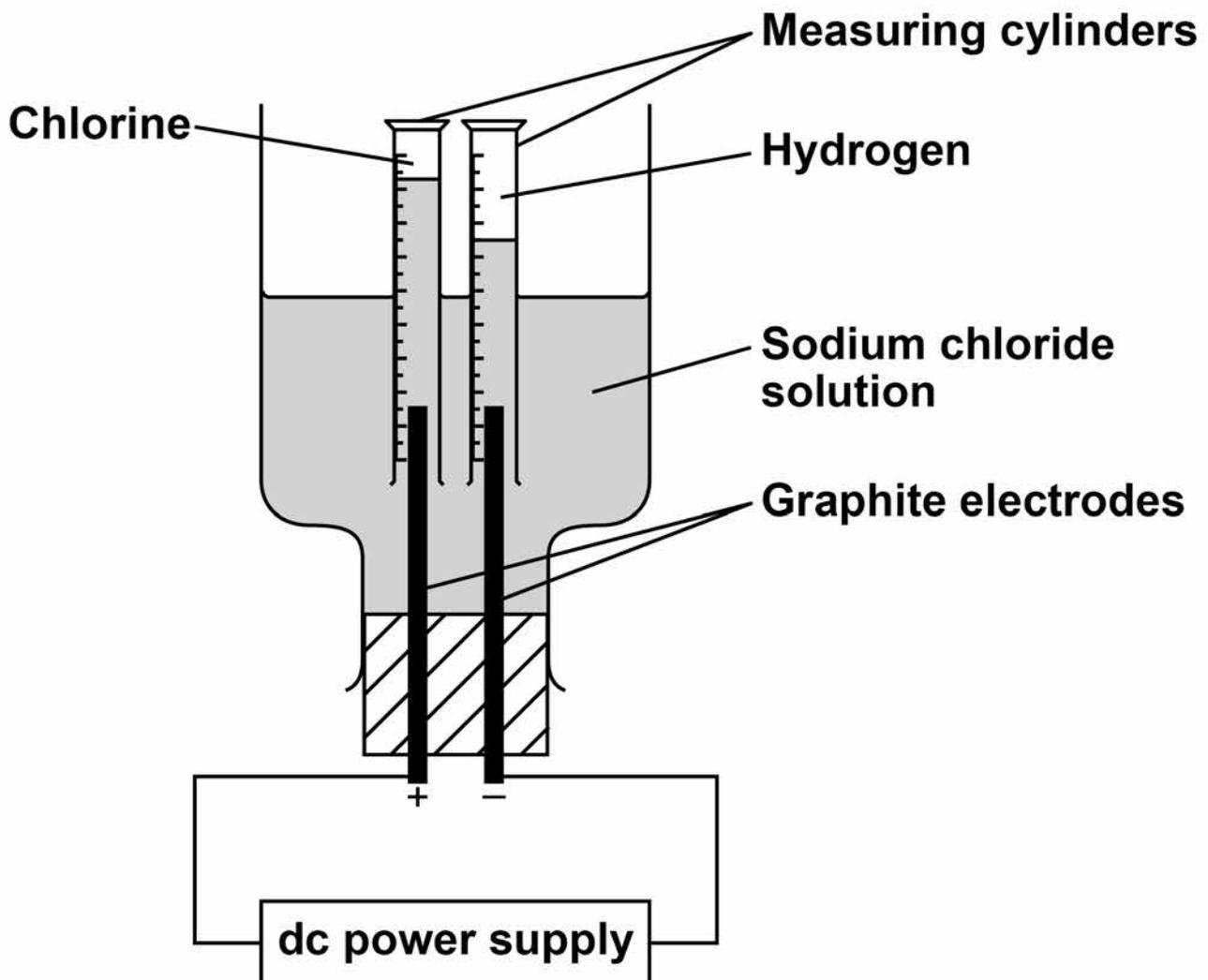
The student measured the volume of gas collected in each measuring cylinder every minute for 20 minutes.
