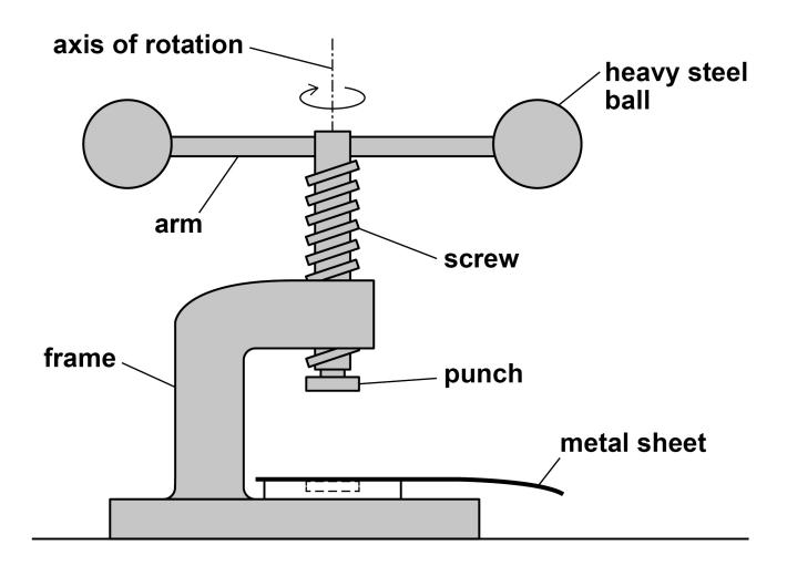
The frame holds a screw and punch. Two arms are attached to the screw, each loaded with a heavy steel ball. The screw is driven downwards when the arms are rotated.
