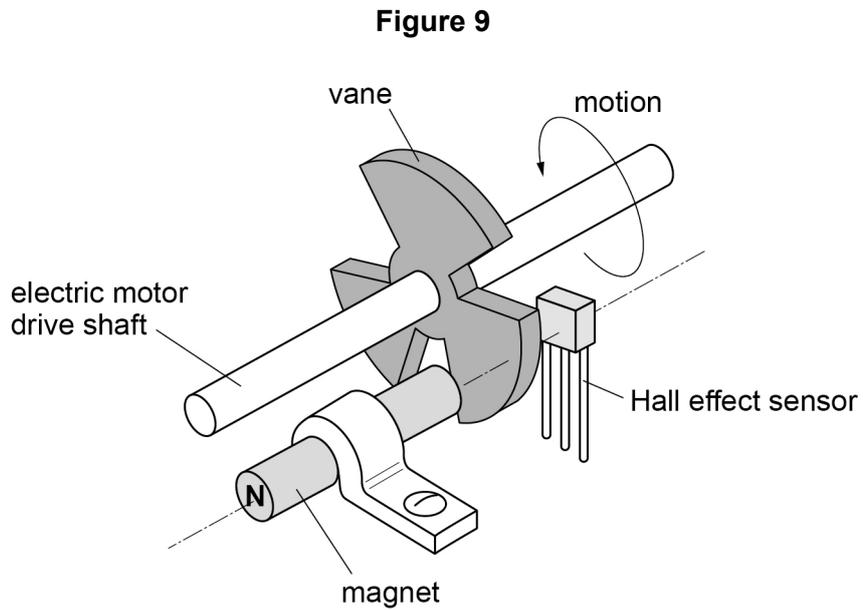
The output of the Hall effect sensor is connected to an oscilloscope. When the vane is between the magnet and the Hall effect sensor, the output of the Hall effect sensor is low.
