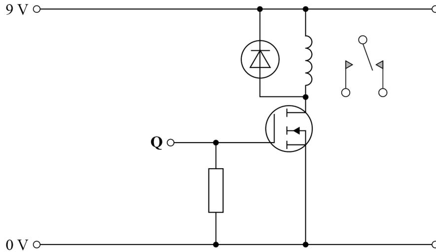
The circuit uses a MOSFET to activate a relay.
