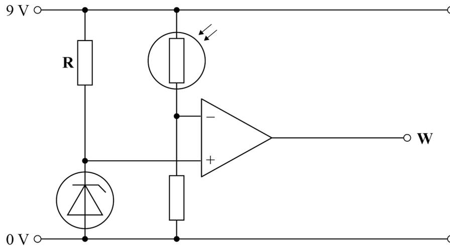
State the function of the Zener diode in this circuit.
