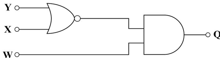
Write the Boolean algebra expression for the output **Q** in terms of **W**, **X** and **Y** based on the logic gates shown in **Figure 13**.
