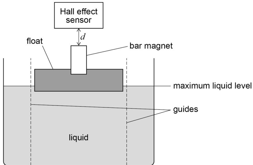
The Hall effect sensor produces an output voltage  $V$ .  $V$  depends on the distance  $d$  between the sensor and the magnet.
