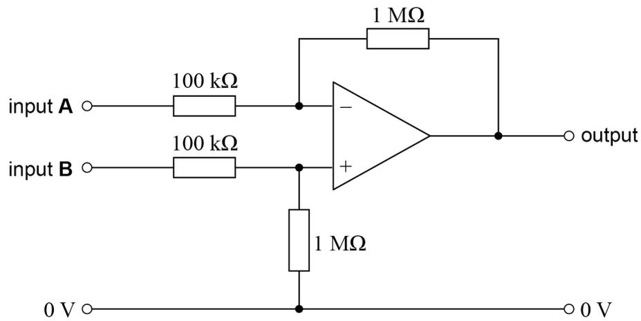
The power supply for the amplifier is  $-12\text{ V}$  and  $+12\text{ V}$  but this is not shown in Figure 4.
