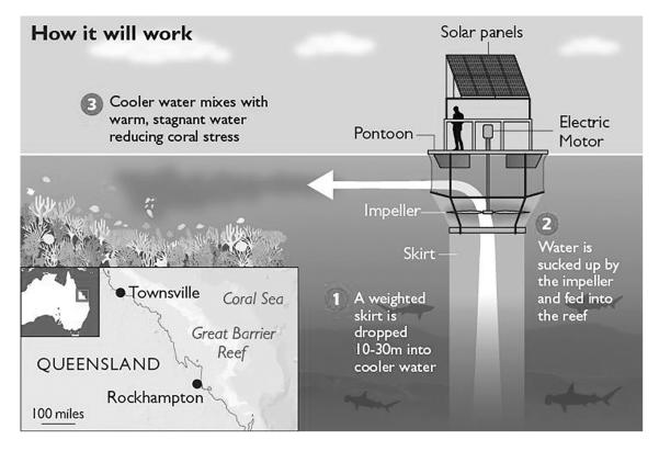
The machines, mounted on pontoons, use large rotating pumps to draw cooler water from 30 metres below the surface and propel it over the coral to re-create cold currents around the reef that have been weakened by warming seas. The cooler currents reduce damage and help the reef to recover after warmer water has bleached the coral.
