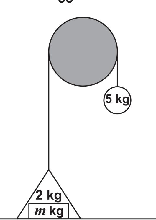
The mechanism is released from rest, and the container begins to move upwards with acceleration  $a\,\mathrm{m\,s}^2$
