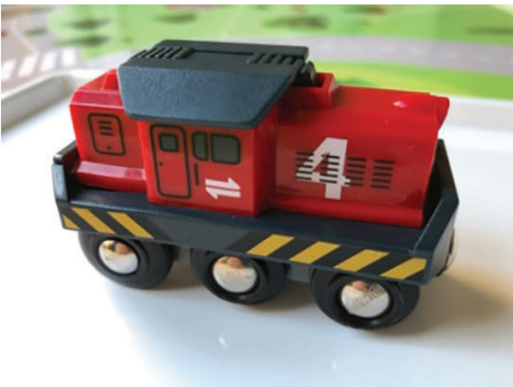
FIGURE 9 Acrylonitrile Butadiene Styrene (ABS) toy (injection moulded)
