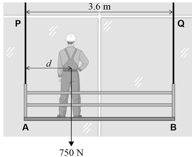
The platform weighs 1800 N and is suspended by vertical cables **P** and **Q**. Each cable has an unstretched length of 3.0 m. The horizontal distance between **P** and **Q** is 3.6 m.
