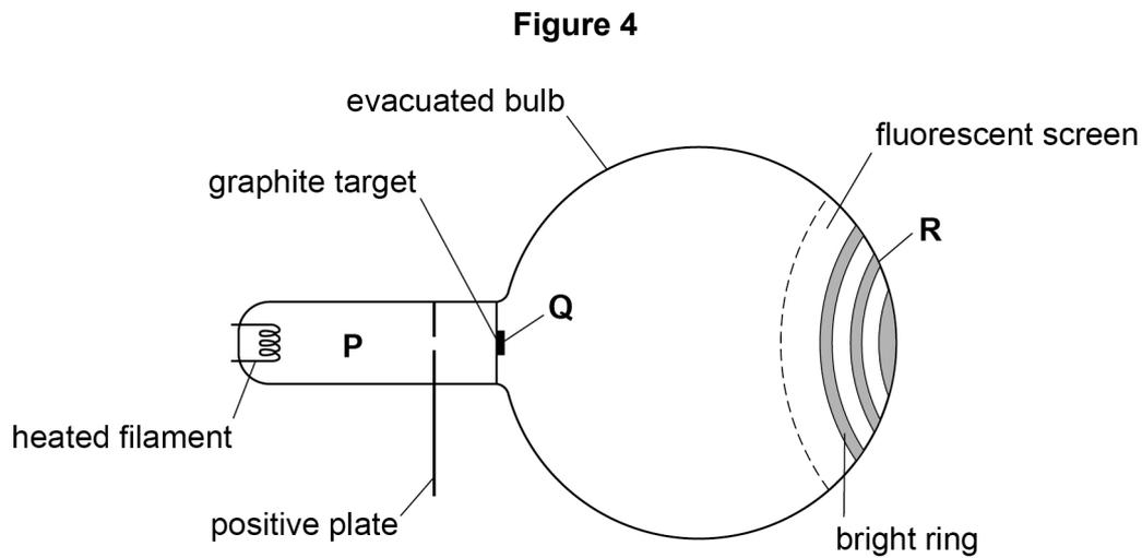
The heated filament emits slow-moving electrons.
