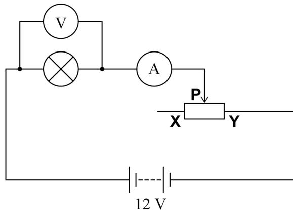
The position of **P** is adjusted so that the reading on the voltmeter is at its minimum value of  $0.75 \text{ V}$ .
