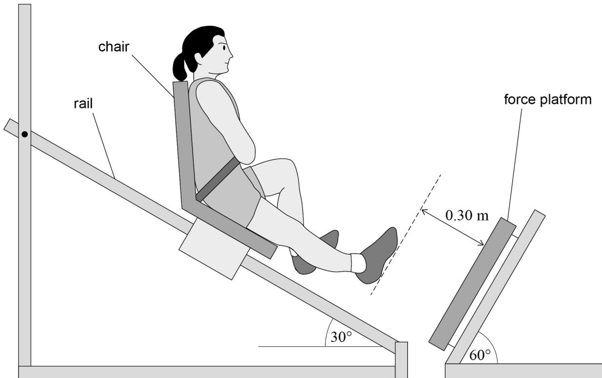
In **Figure 6**, the athlete is strapped into a chair and held at rest halfway along a rail. The chair is then released to slide down the rail. The athlete keeps her right leg extended until her right foot makes contact with a force platform. Friction between the rail and the chair is negligible.
