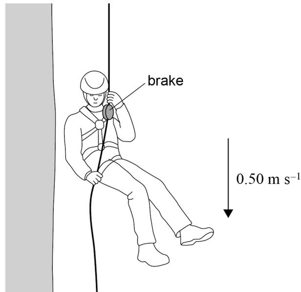
The climber uses the brake to descend at a steady speed of  $0.50 \text{ m s}^{-1}$ . The combined mass of the climber, the harness and the brake is  $60 \text{ kg}$ .
