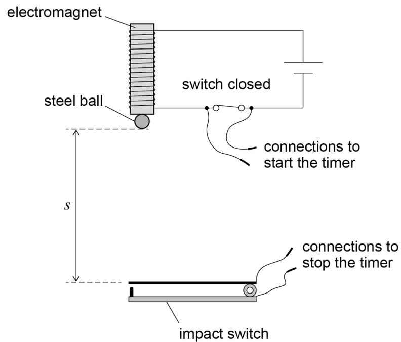
When the switch is opened a timer starts and a steel ball is released from rest. The ball falls vertically onto an impact switch and this stops the timer. The timer displays the time  $t$  for the ball to fall through the vertical distance  $s$  shown in **Figure 1**.
