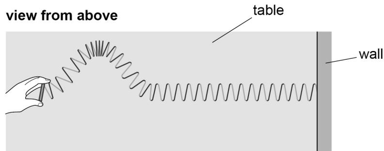
The free end of the spring is quickly moved to one side and then back to the centre, creating a pulse.
