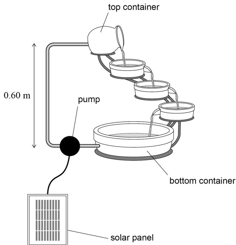
Solar energy is incident on the solar panel at a rate of 1.5 W.
