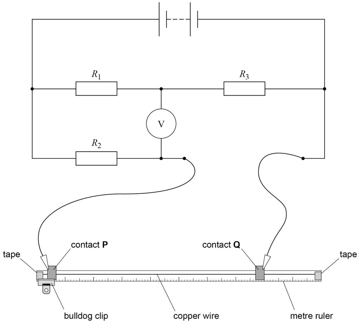
The copper wire is fixed with tape to a metre ruler that has 2 mm graduations. Contact **P** is placed on the wire close to one end of the ruler and held firmly in place using a bulldog clip. When contact **Q** is placed on the wire as shown in **Figure 3** the voltmeter shows a non-zero reading.
