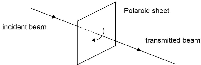
The Polaroid sheet is rotated about the beam by  $90^\circ$  and the intensity of the transmitted beam decreases to zero.
