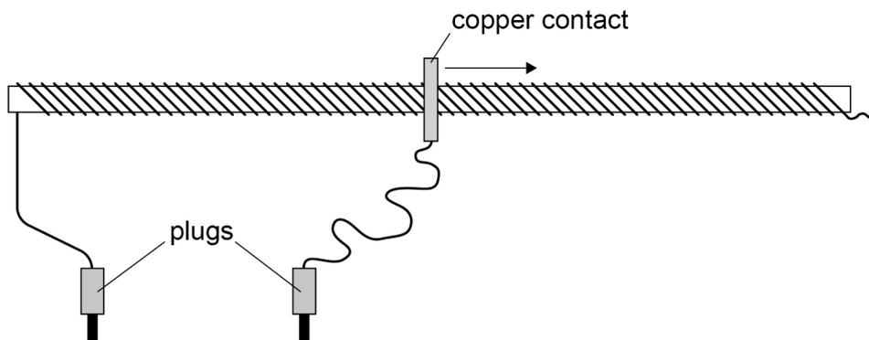
Two plugs connect the variable resistor into the circuit. A moveable copper contact is used to vary the length of wire in series with the lamp.
