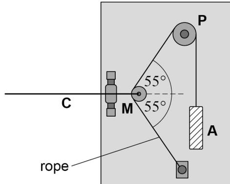
Pulleys **P** and **M** are frictionless so that the tension in the rope attached to **A** is equal to the weight of **A**.
