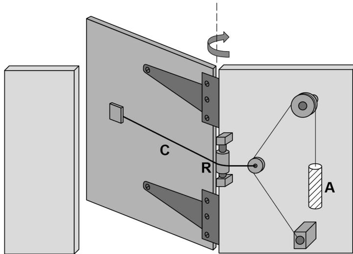
The pulley system raises weight **A** when the gate is opened. When the gate is released, **A** falls. The horizontal cable **C** passes over pulley **R**. The tension in cable **C** causes the gate to close.
