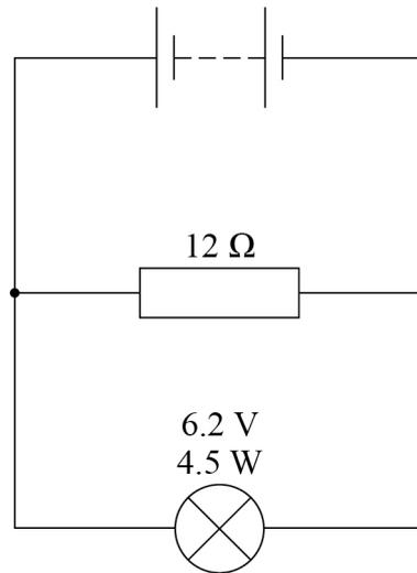
The battery has an internal resistance of  $2.5 \Omega$ .
