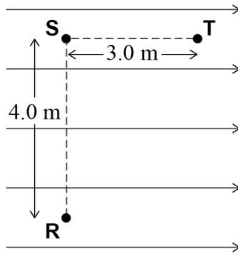
What is the total change in electrical potential energy for a charge of  $3.0 \mu\text{C}$  moving from **R** to **T**?
