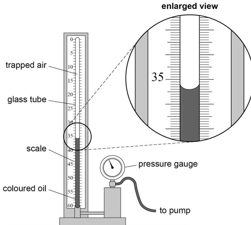
A fixed mass of air is trapped above some coloured oil inside a glass tube, closed at the top.
