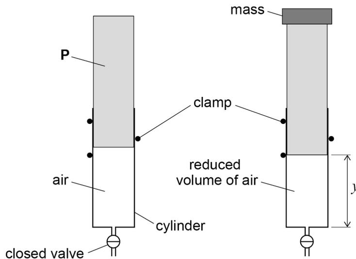
The vertical distance  $y$  between the end of **P** and the closed end of the cylinder is measured.
