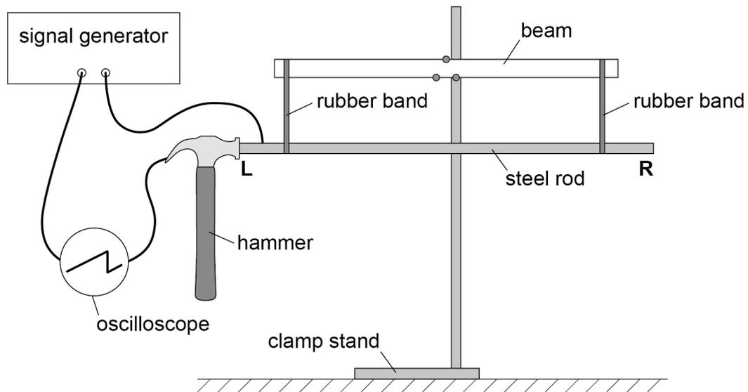
The steel rod is suspended from a beam using rubber bands. When the hammer is in contact with the end **L** of the steel rod, a circuit is completed and the signal generator is connected to the oscilloscope.
