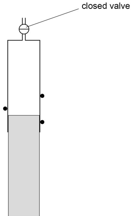
Explain why **P** does not fall out of the cylinder unless the valve is opened.
