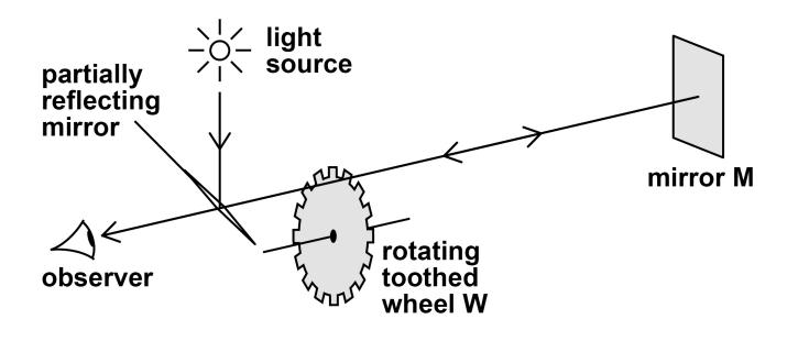
The toothed wheel W is rotated and the reflected light from a distant mirror M is observed.
