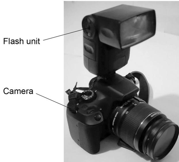
**0 5 . 3** The flash unit emits light from xenon gas in a fluorescent tube.
