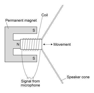
A current in the coil of the loudspeaker causes the coil to move.
