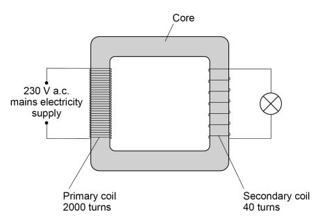
0 8 . 1 What material is used to make the core of the transformer?
