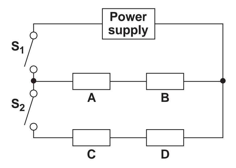
The resistors A, B, C and D represent four heating elements in the hair straighteners.
