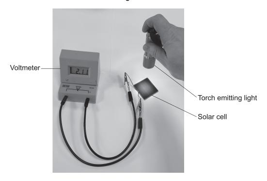
The voltmeter displayed the potential difference generated by the solar cell.
