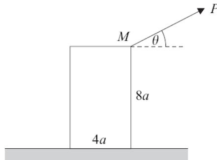
The rope is pulled with a force  $P$ , which acts at an angle of  $\theta$  above the horizontal and is perpendicular to the top edge.
