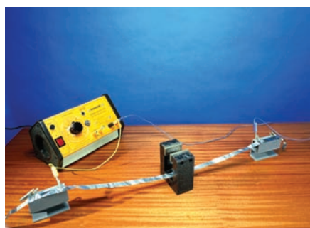
▲ Figure 5.24 The aluminium foil carrying a current is pushed out of the magnetic field.
