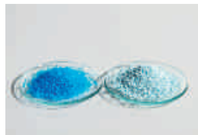
Figure 5.2.8 Blue, hydrated copper sulfate becomes white when heated and the water is driven off
